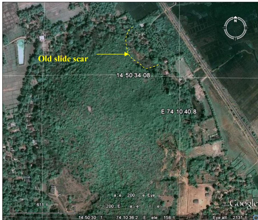
Fig-2: The Google image showing the slope prior to failure and the probable old slide scar
