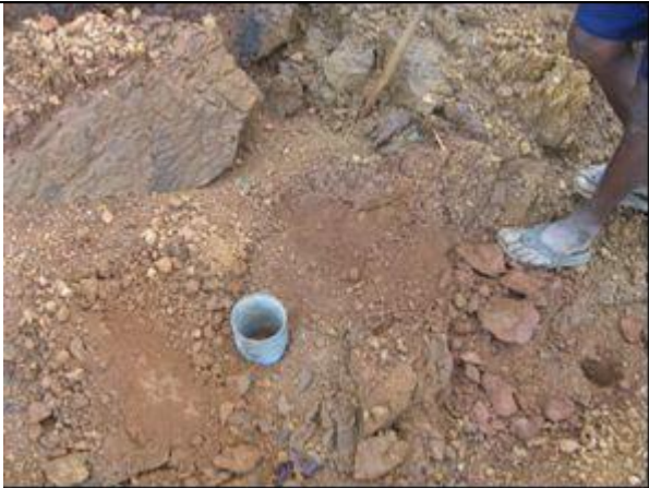
Photo 15: Collection of undisturbed sample (UDS) just below the crown
